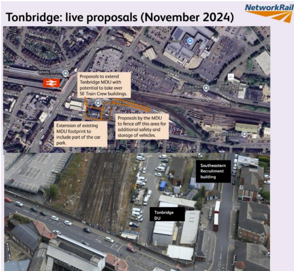
Figure 10 Existing proposals at Tonbridge Station. The photo above gives a close-up view of the area. Source: Network Rail/Google Maps .
