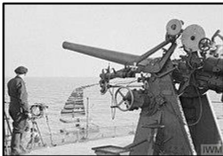
A 3" gun on a ship guarding one of the gates in the anti-submarine net
